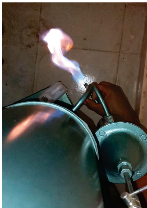
Plate 3. Test for the combustibility of the produced gas
