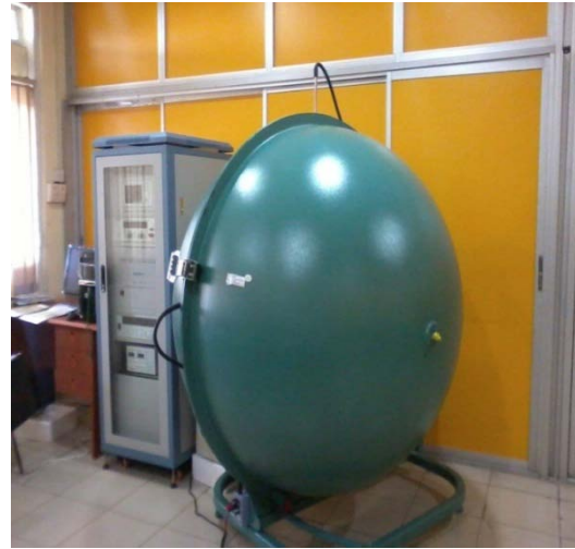
Fig. 3: YF-1000 lamp Testing Analysis Machine at National Centre for Energy Efficiency and Conservation (NCEEC)
