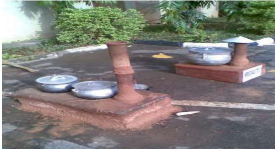
Fig. 8: Double & single -pot energy saving stove by SERC, Sokoto
