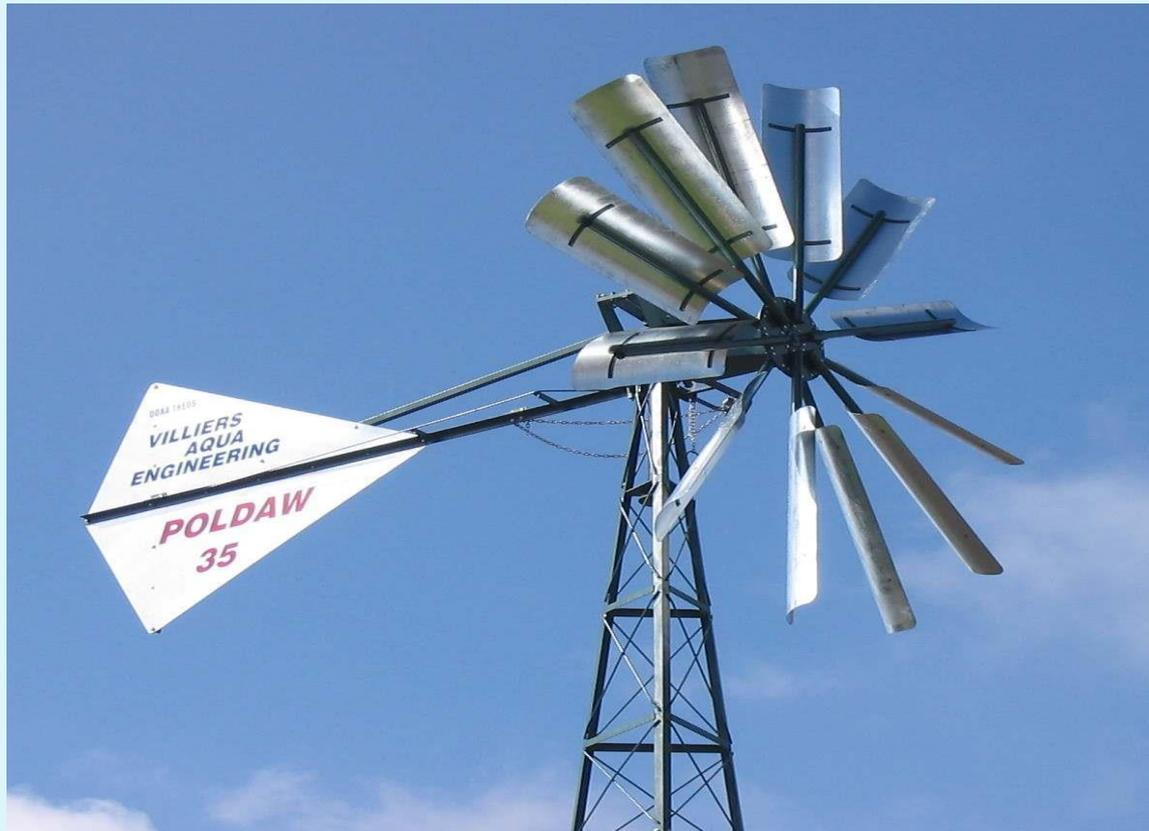
Drag Type wind Turbine for Water Pumping
