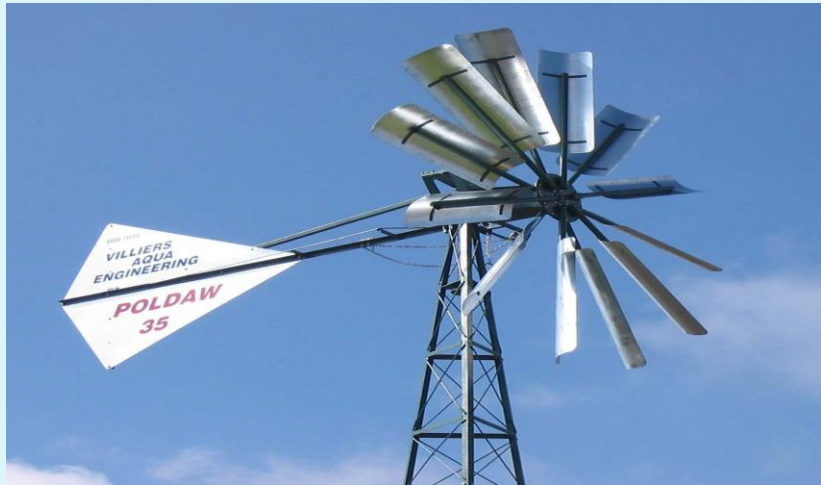
Drag Type wind Turbine for Water Pumping
