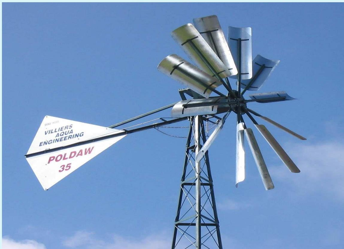
Drag Type wind Turbine for Water Pumping
